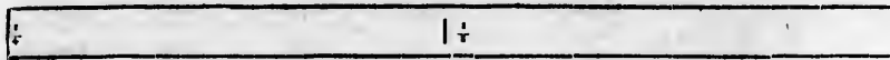
The Length of a Quarter of the Brabant , or Antwerp Aun or Ell, having 6 French Inches and 4\frac{1}{2} Lines.
