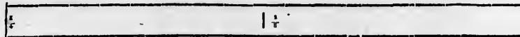
The Length of a Quarter of a Brasse of Venice , for measuring Woollens, &c.
