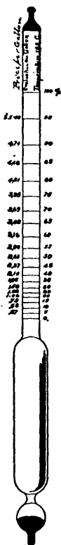
HYDROMETER with moveable price scale corresponding with the percentage of alcohol. Aug. P. Fortin, E. E. P., Montreal.
