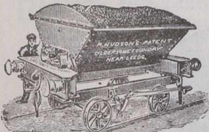
59—R. H.'s Patent 6-Ton Steel Double Side Tip Wagon, to work with ordinary 4-ty Wagons
