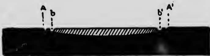
FIG. 12.—Clearing of wood between knife cuts.
