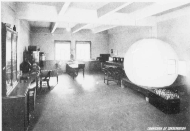
ONTARIO HYDRO-ELECTRIC POWER COMMISSION—PORTION OF LAMP LABORATORY, TORONTO, ONT., SHOWING LARGE PHOTOMETER ON RIGHT.
