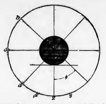
are which s ibtends the angle at the instrument, and this angle will vary inversely with the radius or distance. Therefore at one chain the number of turns of the sorew would be represented by 40 n=N. If now the rod be held at any unknown distance denoted by X ehains, and the num-
