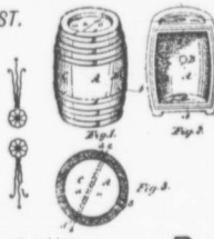
FIG. 1 is an exterior view of Cask. FIG. 2 is an interior perspective view of one section of the Cask. FIG. 3 is a transverse horizontal section through middle of Cask.
