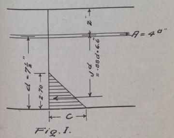
A = 4 sq. ins. =  $\frac{1}{2}\%$  of steel. The unit stress in the steel at No. 140, due to the live load, according to the Chicago Code, is
