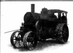
WINDING DRUM ATTACHMENT FOR AVERY DOUBLE UNDERMOUNTED TRACTION ENGINE.
