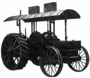
POWER TRANSMITTED THROUGH CONE CLUTCHES One lever controls all speeds and reverse.
