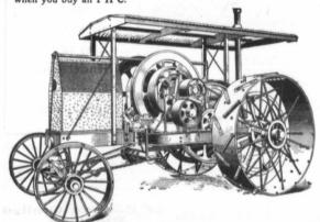
I H C TRACTORS do not require a licensed engineer, nor men and teams to haul coal and water. There is no time lost waiting to get up steam. weight of these tractors is much less than that of steam outfits of equal horse-power and consequently they can be taken over bridges where it would not be safe to take a steam outfit.
