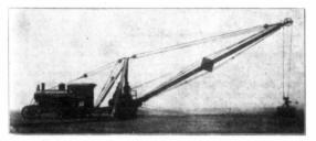
STEAM SHOVEL AND CRANE ATTACHMENT FOR THE AVERY UNDERMOUNTED TRACTION LOCOMOTIVE.
