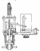
'A' is the piston which moves freely in the cylinder 'C.' The cylinder is in two parts, a small space being left between the two forming a jacket. The hot gases being around and in the inner barrel keep it at an even temperature, insuring practically the same expansion as that of the piston, preventing it from binding at any time. The piston in this particular make of indicator is not straight along the sides but is in the form of a section of a sphere. This insures a line contact be-
