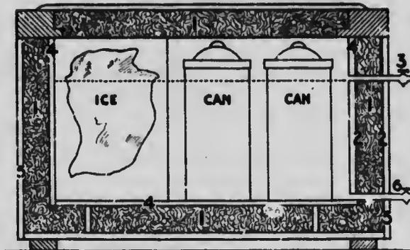
1—Mill Shavings 2—Two-ply damp-proof paper. 3—Overflow water-line. 4—Inner tank made of 1/2 inch lumber. 5—Outer shell of 1 inch lumber. 6—Bottom outlet.
