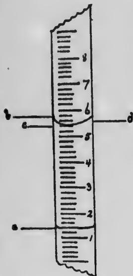
9. It is advisable to use a pair of dividers or compasses for measuring the fat column. The points should be placed at the upper and lower limits of the column to get the length, and then place one point at zero, and the position of the other point will show the percentage of fat in the sample tested. The accompanying illustration will show the correct method of reading milk tests when the fat is at 130° to 140° F. Correct reading A to B, not C or D. For cream, read from A to C.
