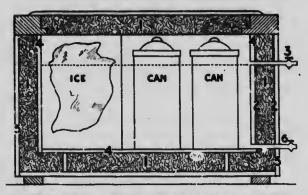
1—Mill Shavings 2—Two-ply damp-proof paper. 3—Overflow water-line. 4—Inner tank made of 1 inch lumber. 5—Outer shell of 1 inch lumber. 6—Bottom outlet,
