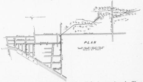
small a portion of the village as possible will be inconvenienced. The valves on the reservoir supply system are so arranged that in the event of emptying the reservoir the coffer dam can be shut off, and in cleaning or repairing the reservoir the water can run from the coffer dam to the village, which, although not being of any great utility, will keep the village from going dry. All valves are provided with cast-iron covers.
