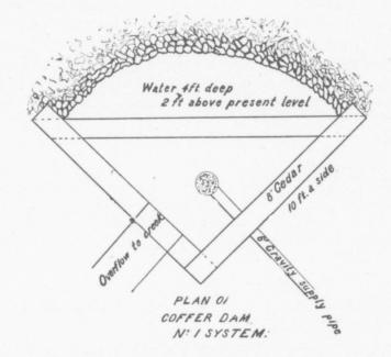
The 6" and 4" supply pipe to the reservoir is laid to a grade sufficient to discharge not less than fifty gallons per minute up to a depth of eight feet of water in the reservoir, which, after that height is reached, gradually fills until the level of the coffer dam is reached.
