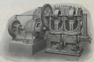
Surface Condenser with 2-throw Edwards Air Pump and Centrifugal Circulating Pump
