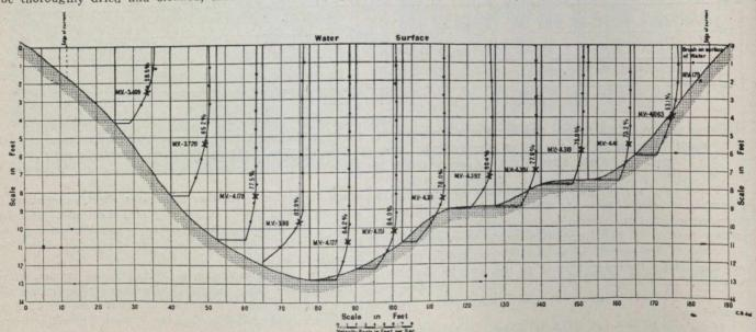
Metering Station on the Montreal River at 1½ Miles above Cillies' Depot showing Vertical Velocity Curves obtained by Measurement made on the 9th of June, 1910. Area of Cross-section 1,482.05 sq. ft. Mean Velocity, 3.94 ft. per Second. Flow, 6,000 C.F.S. Average Depth of Mean Velocity below the Surface = 75.1 per cent.
