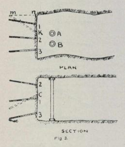
cleaned up, the placing of Fig. 2 (a) is a favorite. Here the adjustable arm is unnecessary and the first setting of the bar is at A to drill the upper and middle rows with the machine above the bar. The second setting of the bar is at B and the machine is turned under it for drilling the bottom row 3 of lifters. The horizontal rows of holes are usually fired in the order 1, 2, 3, Fig. 2 (a).
