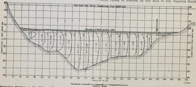
Metering Station on the Ottawa River at North Timiskaming showing Vertical Velocity Curves Obtained by Measurement made Through Ice on the 5th of March, 1910. Area of Cross Section, 5,850 sq. ft., Mean Velocity, 0.771 ft. per. Sec. Flow, 4,510 C.F.S. Average Depth of Mean Velocity Below the Surface = 15 % and 74.5 %.
