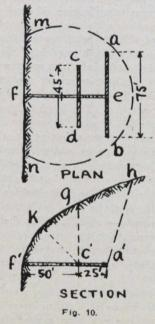
prepare for the corner shots. When the undercut, however, is made by a chain machine, it is of uniform height of only about 4 ins., and the "buster" shot may not throw the coal outwards. It is then often advisable to place an extra "snubbing" shot at f to flatten down the detached prism abc so that the shots d and c can be made effective without first cleaning out the broken coal underneath.
