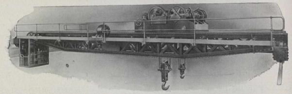
Photograph of 20-ton "Royce" Electrical Crane.
