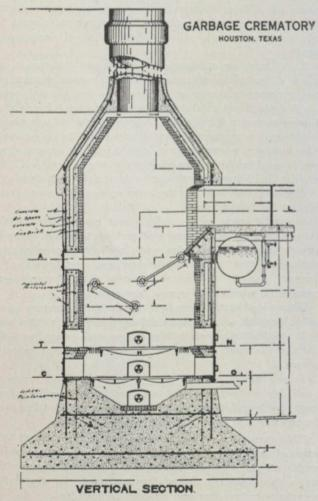
The second compartment is the room between the secondary and main grate. Here the cinders and ashes which have passed the fires above and have dropped through the main grate are reburned before they finally pass into the ash-pit, and therefore absolute combustion must take place. This chamber is also provided with all the necessary regulators.
