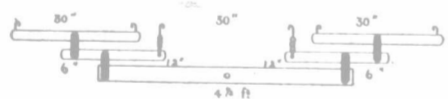
Three-horse Evener, for harrows, plow, or any implement without a tongue.—W. M.
