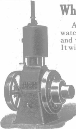
A 2-h.p. Air-Cooled Premier will pump the water for 40 cattle from a well 50 feet deep, and will use but a gallon of gasoline a month. It will drive a 12-in. cutting-box or a wood saw.
