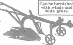
The rod grating is hinged at the front and is given an up-and-down shaking motion by the sprocket wheel at the rear. This shakes the dirt from the tubers and leaves them clean and whole on the top of the ground.
