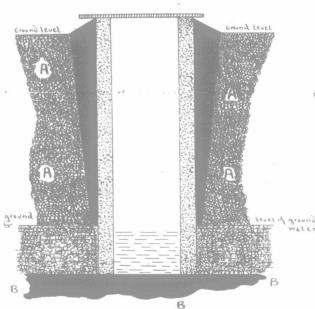
Diagram of well, showing a backing of puddled clay or other impermeable materials between the cementwork and the porous strata through which the well is dug.
