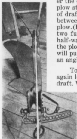
Fig. 9—The white line stretching forward over the top of the beam shows the line of draft.
