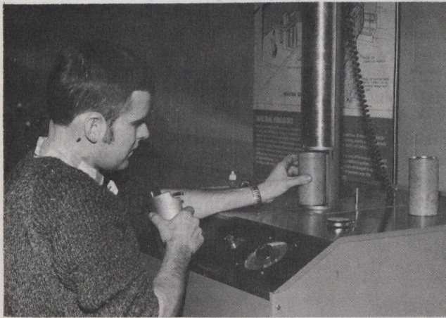
Technician John French places budworm moths in a Gammacell unit. The irradiated males will be able to mate with females but there will be no offspring.
