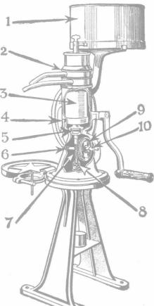
9 Worm wheel clutch stops all mechanism when crank is stopped, with exception of bowl and worm wheel. No lost motion in again starting crank as clutch grips instantly and without jar to the mechanism.
