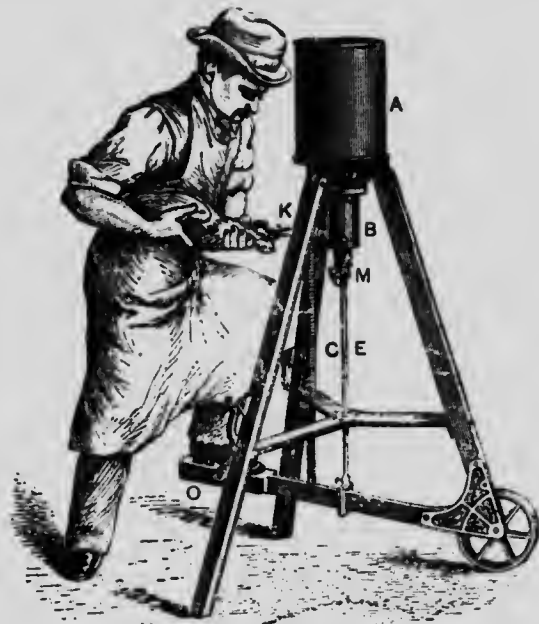
Fig. 51. Cramming Machine for Forced Feeding of Chickens, Turkeys, etc.
