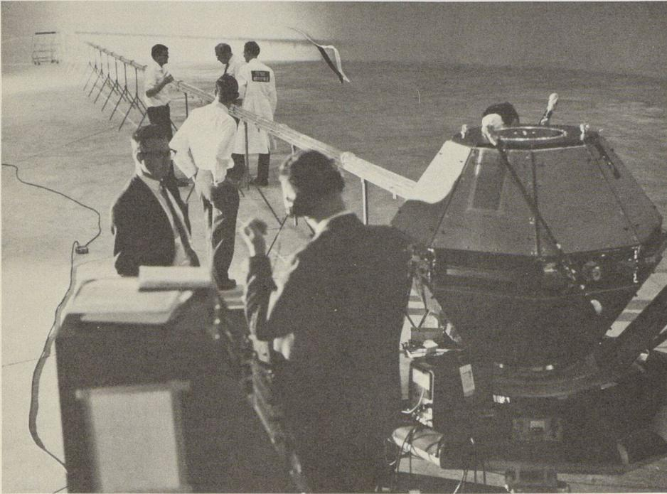
One of two 240-foot antennae on ISIS A being tested prior to launch last January. In orbit, these NRC developed antennae uncurl like steel measuring tapes. They are on all Canadian satellites and were used on the U.S. Gemini space craft.
