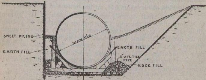
TYPICAL SECTION OF PIPE TRENCH IN EARTH
