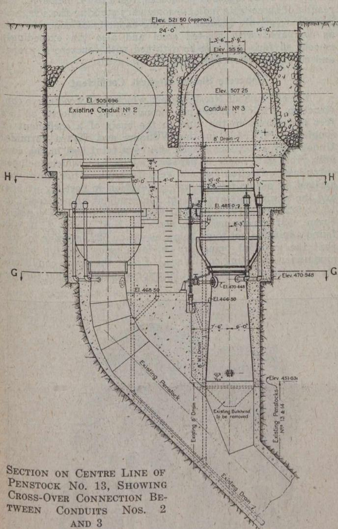
SECTION ON CENTRE LINE OF PENSTOCK NO. 13, SHOWING CROSS-OVER CONNECTION BETWEEN CONDUITS NOS. 2 AND 3
