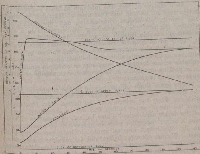
SURGE TANK STUDY FOR FULL LOAD REJECTION, CONDUIT No. 3
