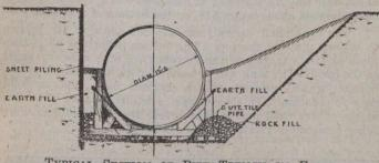
TYPICAL SECTION OF PIPE TRENCH IN EARTH
