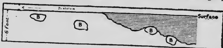
Figure 3. Diagrammatic vertical section showing contact of stratified Leda clay (shaded) with boulder clay (unshaded), near Pointe Claire. B = Large boulders. Length of section 50 feet.
