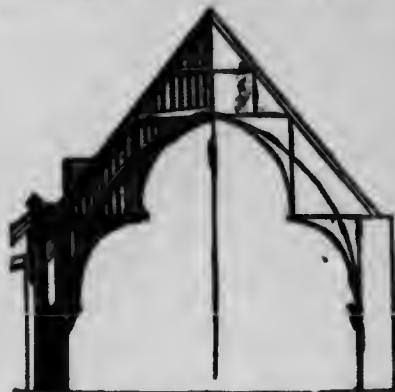
Hammer-beam Roof, Westminster Hall.
