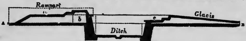
Section through Line of Fortifications.
