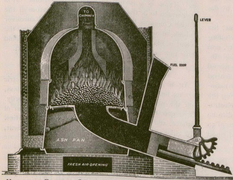
UNDERFEED FURNACE—SECTION SHOWING METHOD OF INTRODUCING FUEL.
