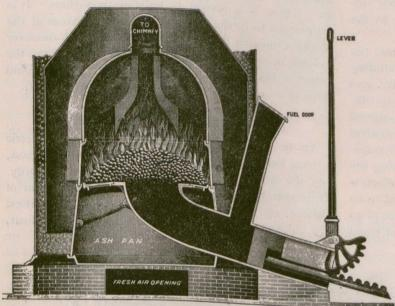
Underfeed Furnace—Section Showing Method of Introducing Fuel.
