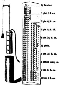
Having placed the smaller vessel perfectly upright, measure into it a gallon of water less half an ounce, and with a rule ascertain the precise distance from the surface of the liquid to the brim of the vessel, then placing this measure outside of the tin, mark the height of the water as 230 c. in. In a similar manner with half a gallon and 101 fluid ounces, mark 134 c. in.
