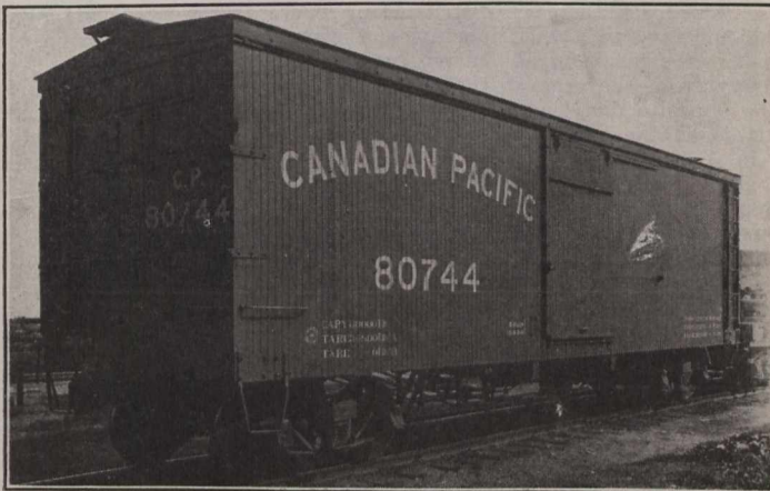
Fig. 1.—C.P.R. Steel Centre Sill Wooden Box Car.
