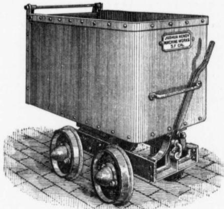
wheels in turn running loose on the axles. This method of construction makes them very easy running. The cars are made in four sizes of 1,000 lbs., 1,200 lbs., 1,600 lbs. and 2,000 lbs. capacity, respectively. They are manufactured and kept in stock by the Joshua Hendy Machine Works, of Nos. 38 to 44 Fremont street, San Francisco, the well-known manufacturers of high-grade quartz mining and milling machinery, who will furnish catalogues and prices upon application.
