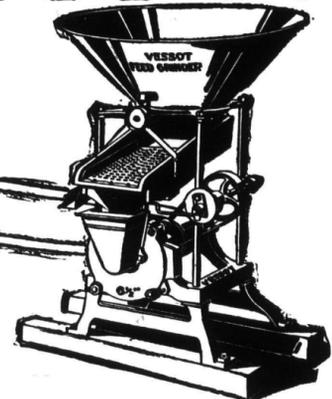
THE Vessot "Champion" cleans grain as well as grinds it. The spout that carries the grain to the grinder is made with two sieves, a coarse one above and a fine one below. The coarse sieve catches nails, sticks, and stones, but lets the grain fall through. The fine sieve holds the grain, but takes out all sand and dirt. The grain passes to the grinding plates as clean as grain can be.
