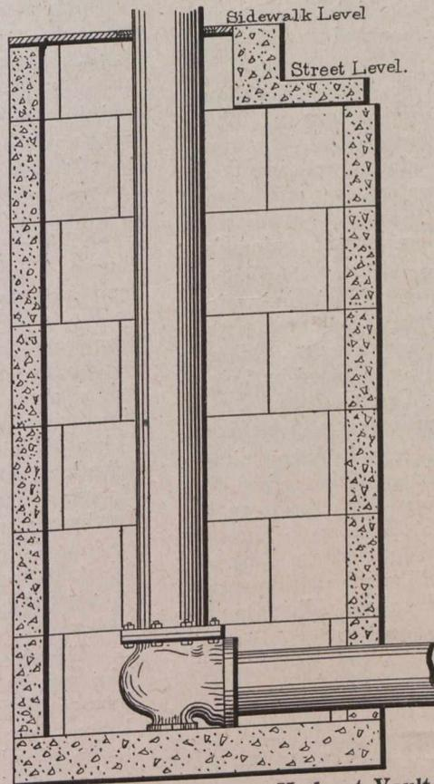
Fig. 3.—Unit-built Fire Hydrant Vault.
