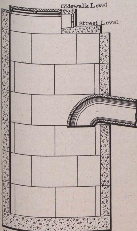
Fig. 2.—Catch Basin Built of Concrete Block Units.
