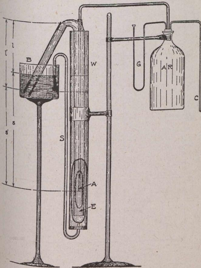
Fig. 1.—Model of Air Lift Pump.
