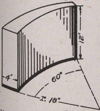
Fig. 1.—Concrete Block, Unit of Construction.
