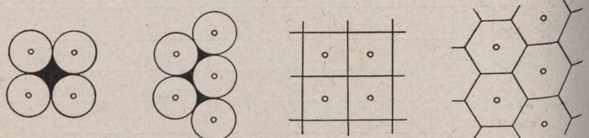
Fig. 2.—Areas Covered by the Different Shaped Nozzles.
