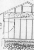
Fig. 3.—End View Shows gable roof with thatch that the straw extends to meet foundation walls at 10 inches above the concrete
