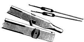
ting these up, the handles are kept about  $\frac{1}{2}$  in lower than wanted, and firmly bolted into the ratchets on the mouldboard and head, then with the use of the buckles the desired height and tension on the rods is secured. All the parts are held perfectly rigid and are not liable to shake loose. This valuable improvement is used on all "Verity" Plows.
