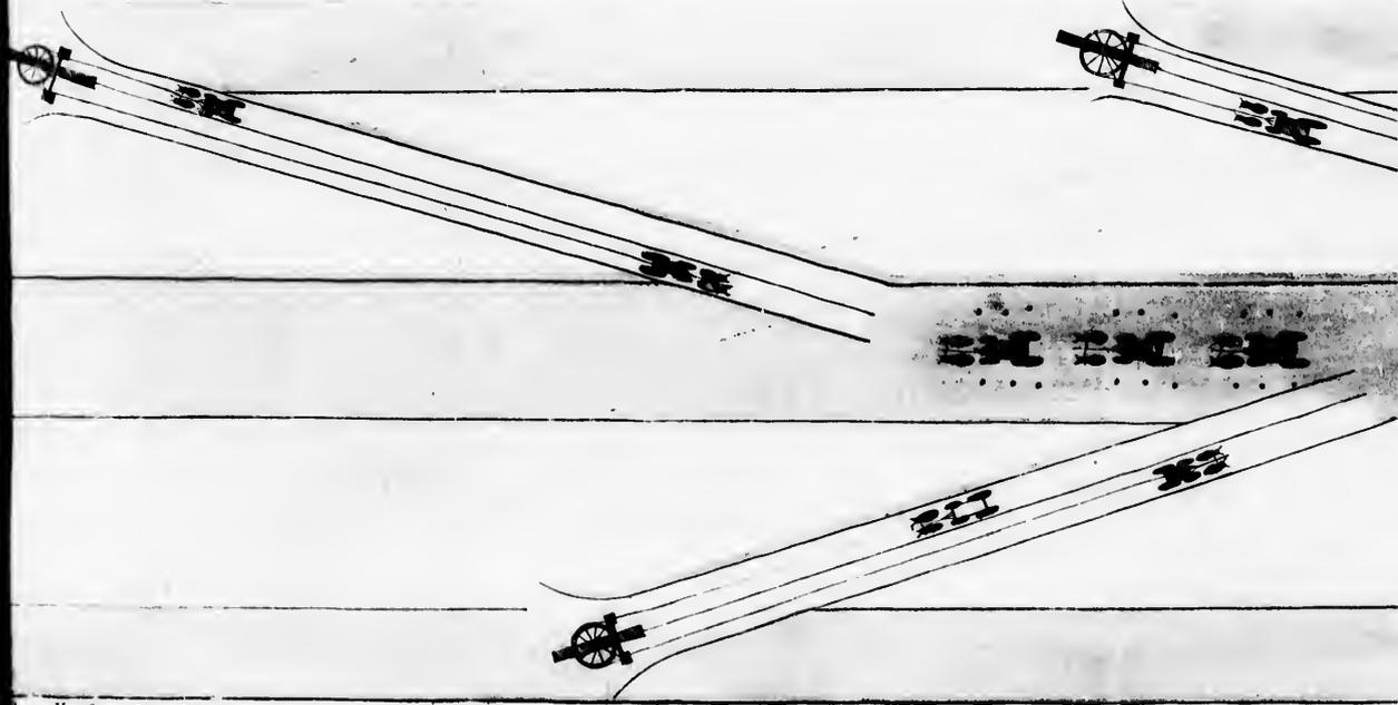
*Moving Earth in deep Cutting - as seen in profile from the bottom of the Canal* By O. Phelps
