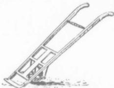
will mount a wheel beneath a frame, as shown in the cut, and the frame ought to be within the ability of anyone handy with tools. A medium-sized, single-wheeled truck will do much work, and do it easier than is possible with a small, double-wheel truck.
