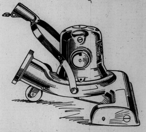
The Ohio Vacuum Cleaner has but two necessary oiling operations-one directly at the top of the motor and the other at the bottom. The oil is absorbed by two large felt pads which will prevent over-oiling, splashing and dropping of oil on the carpets.
