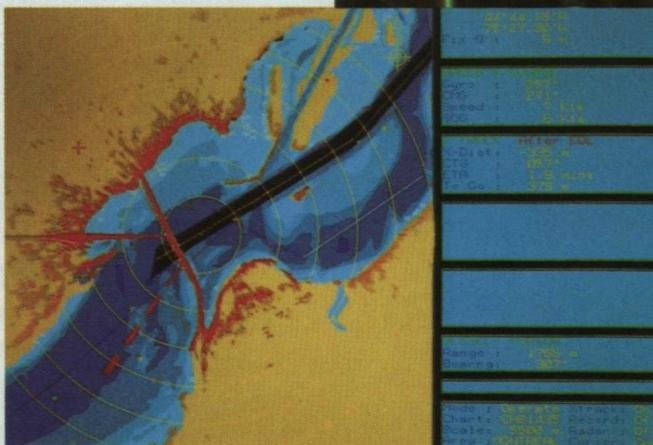
Working electronic charts with real-time display of ship's position have been developed by QSL. Here, matching of chart and radar image overlay eliminates most position ambiguities.
