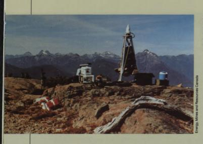
A satellite Global Positioning System (GPS) site and receiving antenna centred over a geodetic marker.
