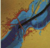
Working electronic charts with real-time display of ship's position have been developed by QSL. Here, matching of chart and radar image overlay eliminates most position ambiguities. PROCOM-2, a geographic information system developed by Gregory Geoscience, projects a Landsat image onto a map for interpretation by analysts. 13
