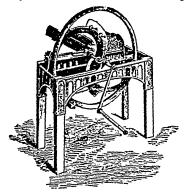
The above cut represents a machine with two knives, simple in construction, neat in appearance, expeditious in operation, portable and effective for its purpose, and produces a clean and neat cut. It can readily be fed and turned by one man, and cuts easily 20 bushels an hour. Price  $\pounds 4$  10s. Extra knives 4s. 6d. each.
