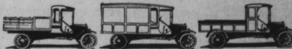
Three of the many body styles that may be mounted on the Ford truck chassis
