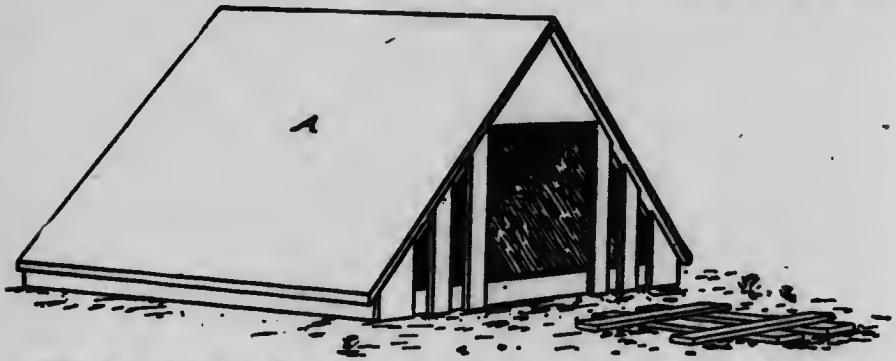
Fig. 16. Coop A.—Each side of roof 24 in. by 30 in.; bottom 2 ft. 4 in.
