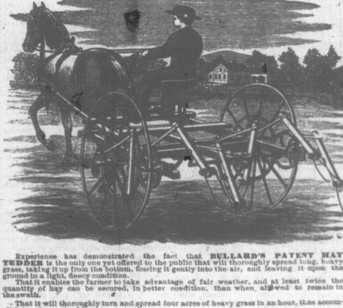
Experience has demonstrated the fact that BULLARD'S PATENT HAY TEDDER is the only one yet offered to the public that will thoroughly spread long heavy grass, taking it up from the bottom, tossing it gently into the air, and leaving it upon the ground in a light, feecy condition.
