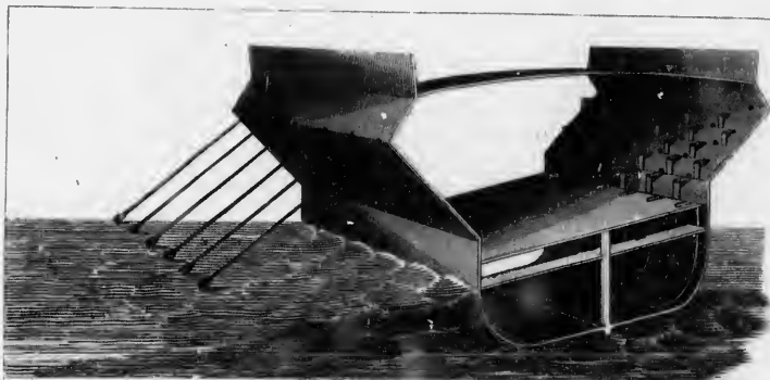
A perspective view of part of the waste of an ancient war Galley of five the position of the benches and oars, as explained by GENERAL MELVILL
