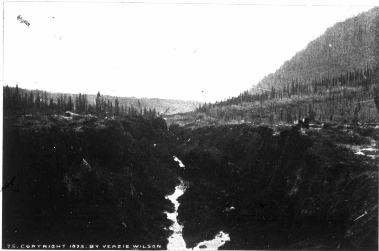
GROUND SLUICING. This is done without any sluice boxes, the water being turned right on the ground, washing away the dirt and leaving the gold.
