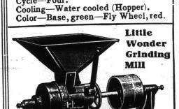
Especially adapted for gasoline engines. Most successful little grinder in the world. Made of iron and steel and has few wearing parts. It is not liable to get out of order. Will run empty without in jury to burs. Grinds all kinds of grain. Grind from 5 to 15 bushels per hour if run from 600 to 1,200 revolutions per minute. Requires 1 to 3 b.p. to operate. Burs are 5 in.. drive pully 6 in. weight 90 lbs. Price, complete with two sets of burs. \$10.50,
