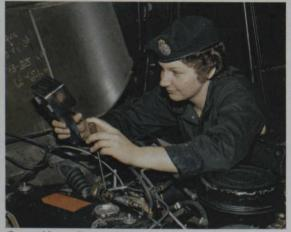
Corporal Lynne Fraser, a Vehicle Technician at Canadian Forces Station Falconbridge, adjusts the engine of a 4 ton truck.
