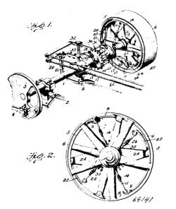
tional shoes carried by the fixed wheel and adapted to frictionally engage the loose wheel and look said loose wheel to the fixed wheel, and means for operating said frictional shoes, substantially as set forth.
