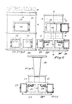
the combustion chamber and ash pits respectively through the jacket and each provided with suitable doors, a smoke pipe and hot air flues leading from the furnace, substantially as described.
