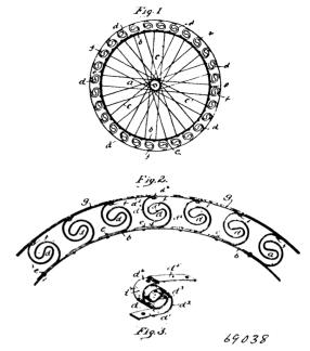
which is reinforced by a continuous band and the outer one of which has its adjacent parts riveted together to form a self-sustained continuous band.
