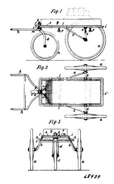
wheel device, comprising the rectangular frame i, the braces n, n, and the braces o, o, substantially as herein set forth.
