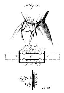
of said plate, salient lips projecting in opposite vertical directions from the upper and lower portions of said bar and teeth extending from said salient lips respectively in the directions thereof.
