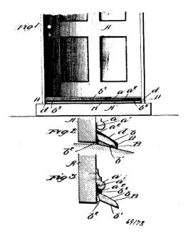
a flange formed on the upper edge of said bracket and adapted to engage said weather strip and hold it in its operative position, substantially as described.
