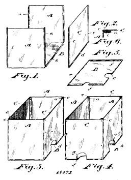
the seams having indentations i, formed therein to prevent the hooked edges pulling apart, substantially as and for the purpose specified.
