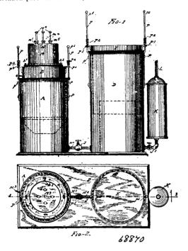
generator cylinder, a receptacle for gas producing material within said cylinder and a closure within said cylinder between the magazine and said receptacle, substantially as shown and described.
