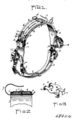
secured to said central strap having their ends turned downwardly forming flanges engaging with the edges of the straps of the holdfast, substantially as described.
