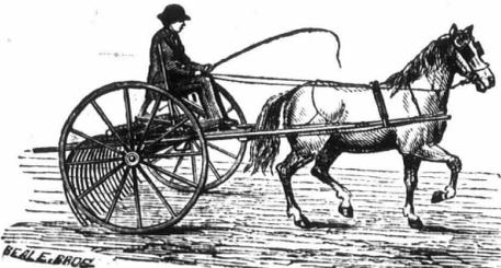
The head is so attached that it permits the teeth to accommodate themselves to uneven ground, the wheels running upon an elevation will not raise the teeth from the ground. By the raising attachment the operator can throw the teeth of the rake higher in passing over the winnow than any other manufactured. The elasticity of the teeth enables it to pass over stones and other obstacles. The teeth are so shaped and attached that they do not scratch or harrow the ground like most steel teeth rakes.
