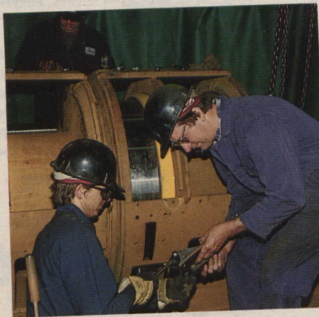
Mechanics at R.A. Warren Equipment Ltd. of North Bay, Ontario complete the remanufacturing of a slusher hoist for export. The company supplies equipment for underground mines in Canada, the US, Latin America and the Philippines.
